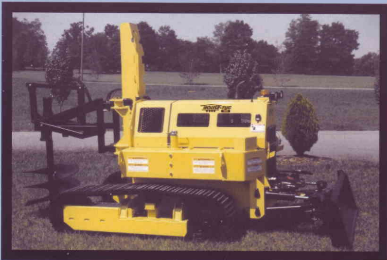
465 SHOWN WITH DOZER BLADE OPTION AND AUGER ATTACHMENT
