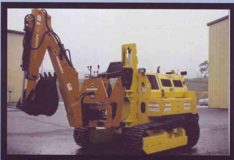
465 SHOWN WITH OPTIONAL BACKHOE ATTACHMENT
