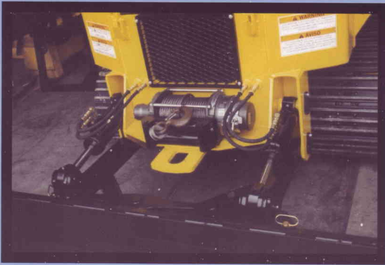
465 SHOWN WITH STANDARD 12,000 LB WINCH AND OPTIONAL DOZER BLADE ATTACHMENT
