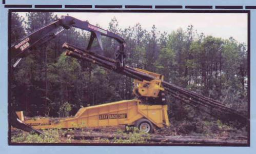
MULTIPLE STEMS BEING LOADED INTO THE PTD-243 PULL-THRU DELIMBER.
