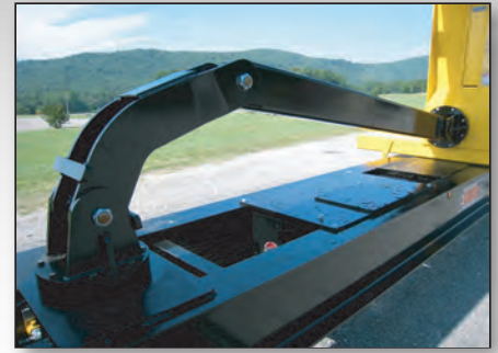
Heavy-duty swing-arm attaches permanently to the loader trailer deck.
