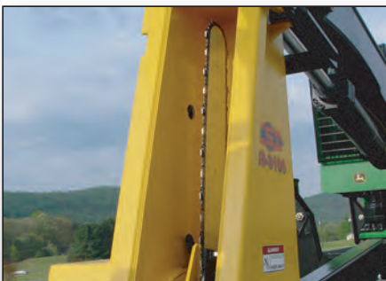
Uses same bar & chain as the PTD-264 Ultra delimeter.
