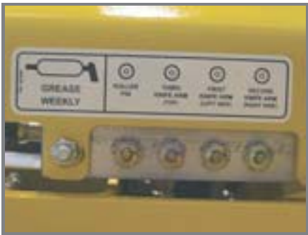
Central Grease Station.
